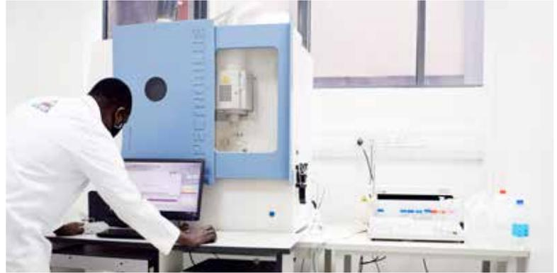
Induction Coupled Plasma Optical Emission Spectrometer ICP OES
